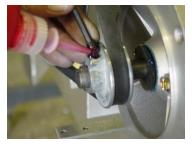
7.) Reinstall set screw and tighten.
