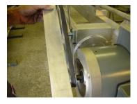
6.) Remove motor pulley set screw. Apply Loctite in hole.
